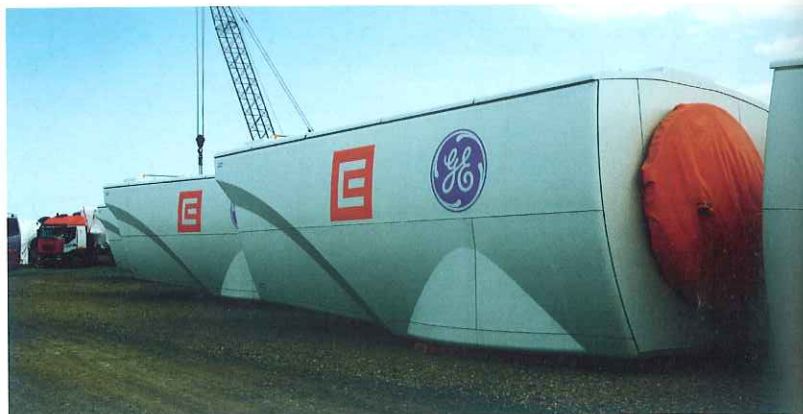
For dispatch GE nacelles heading for the 347.5MW first stage of CEZ's Fantanele-Cogeaalac wind farm
